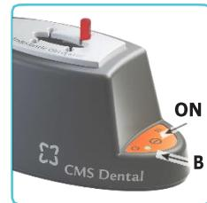
The Heater can be turned off by pressing the ON button for 2 seconds. 3 short beeps indicate that the Heater is turned off. The Heater can be reactivated by pressing the ON button for 2 seconds, by doing so a long beep is emitted.
